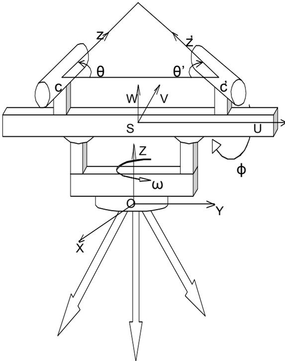
Fig.1 A basic physical structure of Photogrammetron-I
