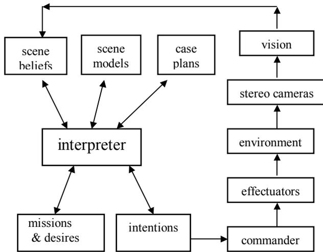
Fig. 2 A reactive BDI agent architecture of Photogrammetron
