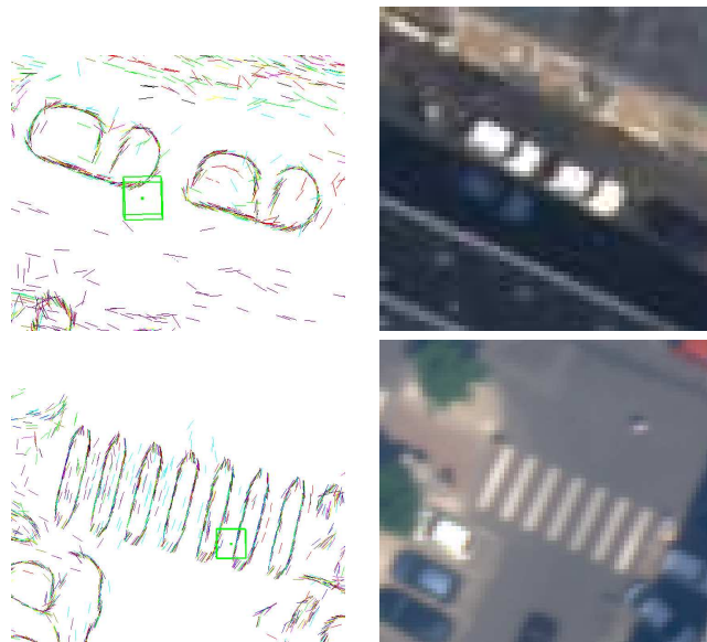
Figure 4: Example of non-linear object extraction with edgels. The shape of small objects (cars, zebra crossing, etc.) are well reconstructed using edgels. The square (upper left and bottom left images) is used as a 1m \times 1m metric reference.
