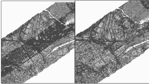
Figure 10. “Model keypoints” in the Gävle project. In the left image are model key points before and in the right after the strip adjustment.
