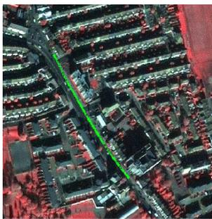
Figure 10. Example of Positioning and radiometric accuracy of IKONOS Precision by k-GPS tracks
