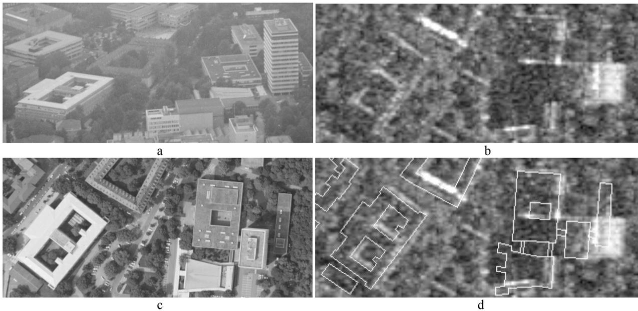
Fig. 6. a) oblique view of the scene, b) SAR image (ground range), c) vertical view, d) SAR image overlaid with the layer BULDING of the vector map. Range direction from right to left
