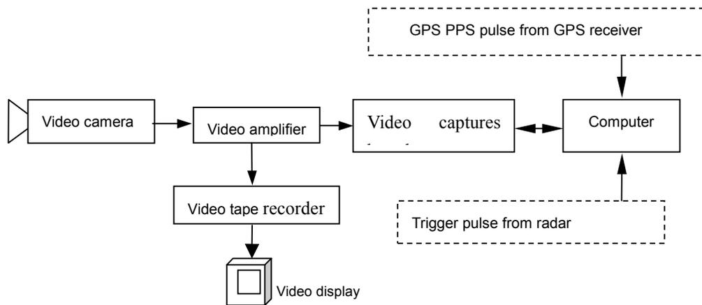
Figure 3. The configuration of video capturing system
