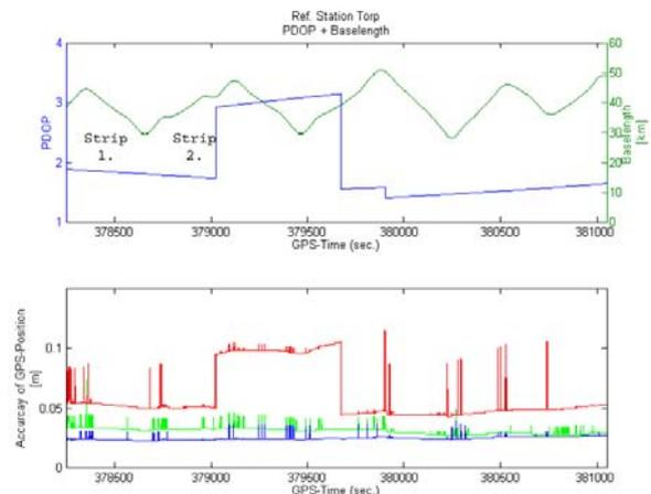
Figure 3: Accuracy of GPS position, reference station Torp
