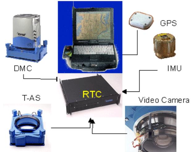
**Figure 3** ASMS Aerial Sensor Management System
