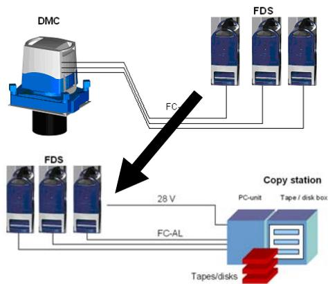
**Figure 6** Flight data storage connected to the copy station
