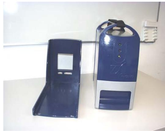
**Figure 5** flight data storage unit FDS
