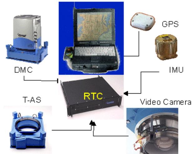
**Figure 3** ASMS Aerial Sensor Management System
