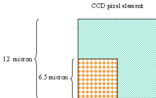
**Figure 4** light sensitive area of a CCD pixel element
