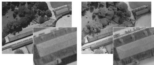
Figure 3: Comparing aerial film and digital image. Left is scanned film at a pixel size of 15  $\mu$ m (GSD of 15 cm); at right is the digital image with a GSD=17cm (from Leberl & Gruber, 2003).
