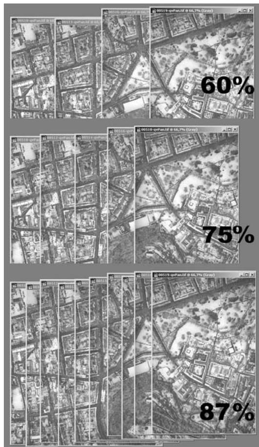
Fig. 2: Sample of a flight line with 60% (top), 75 % (center) and 87 % forward overlap (bottom). This corresponds to a relative base length of 40%, 25% and 13% of the image dimension. The number of frames doubles between each of these examples.
