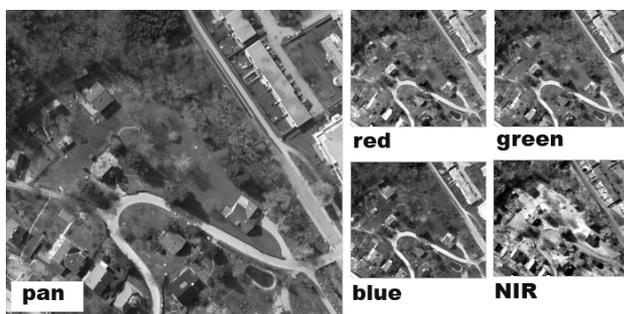
Fig. 4) Panchromatic high resolution image (left) and four multispectral channels (right) built the source data set of UltraCamD.
