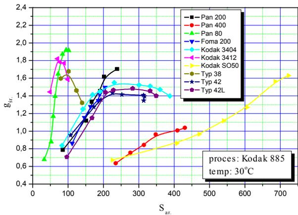
Fig. 6. Graph of relation  $g_{sr}=f(S_{ISOA})$  for films processing in solution 885 at  $T=30^{\circ}C$  in Versamat processor.
