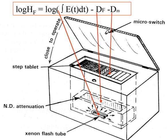
Fig. 1. Diagram of flash type sensitometer /Avisense2000/. [5]
