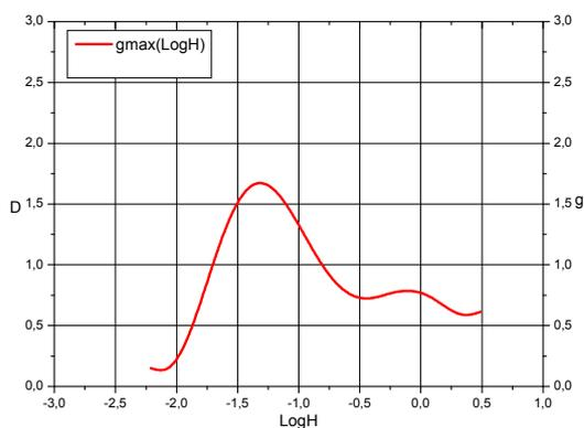
Fig. 9. Distribution of the local gradient  $g = f(\text{Log}H)$  for Agfa Pan 80 film
