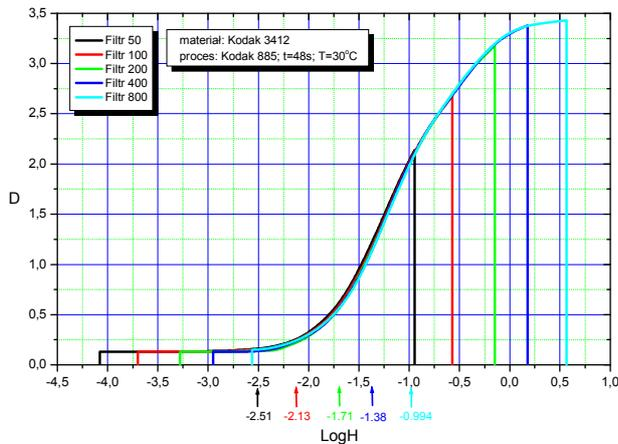
Fig. 3. Characteristic curves of Kodak 3412 material obtained using a set of five filters. In this case, the exposure of  $H=2,13$  lux s ( $\text{Log}H=-1,38$ ) was selected.
