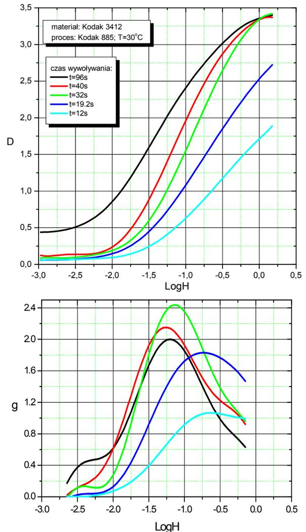
Fig. 5. Impact of the development time on the shape of the characteristic curve and distribution of the local gradient for Kodak 3412 material processed in Kodak 885 ( $T=30^{\circ}\text{C}$ ) process.
