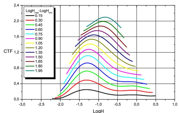
Fig. 11. Courses of Contrast Transfer Function for various values of contrasts of the test ranging from 0.15 to 1.65 determined for Agfa Pan 80 material.
