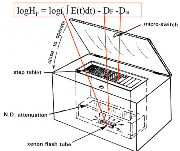
Fig. 1. Diagram of flash type sensitometer /Avisense2000/. [5]
