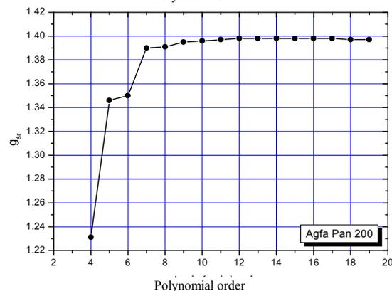
Fig. 7. Dependence of arithmetic photosensitivity ( $S_{ar}$ ) and mean gradient ( $g_{sr}$ ) values on the degree of the polynomial for the Ukrainian material Typ 42 and Agfa PAN-200.
