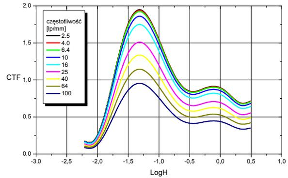
Fig. 10. Contrast Transfer Function graph for spatial frequencies ranging from 2.5 lp/mm to 100 lp/mm determined for the Agfa Pan 80 material
