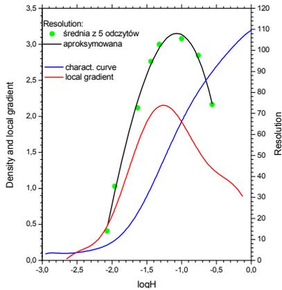
Fig. 8. Graphs of relations  $R=f(\log H)$  and  $g_{max}=f(\log H)$  for the USAF 1951 test exposure of 0,78 contrast and Kodak 3412 film processed in Versamat 1140 processor, AGFA 74,  $v=10$  ft/min,  $T=30^{\circ}C$
