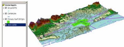
Figure 3a. 3D Visualization of the DSM
