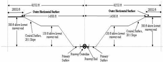
Figure 9. Top View (top) and end view (bottom) of 2D OISs
