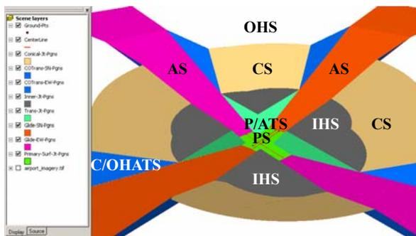
Figure 10b. 3-D View of Draped OIS (Separated Layers)
