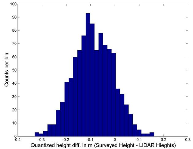
Figure 7: Height differences histogram between the laser height and the ground height.
