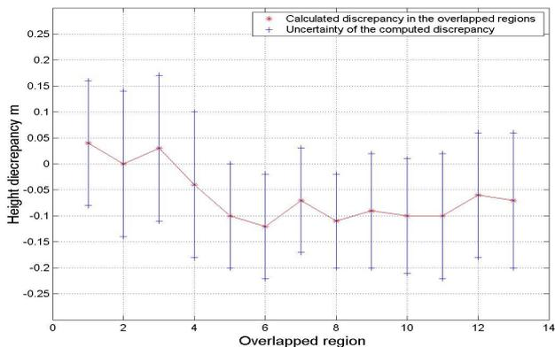
Figure 3: Mean Relative discrepancy behavior between adjacent strips, where the x-axis represents the overlap region (where 1 is the overlap region between strip 1 and 2)
