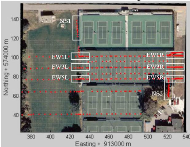
Figure 6: Surveyed ground points over the test area and Selected locations for the planimetric accuracy computation.
