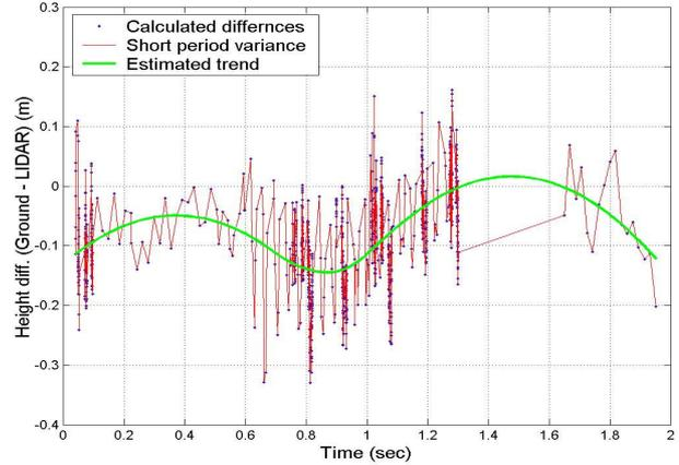
Figure 9: Height accuracy (Ground - LIDAR) versus time.
