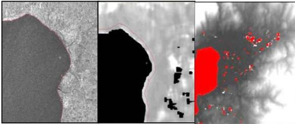
Figure 5 Failed areas and blunders in the extracted DEM
