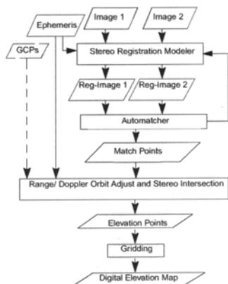
Figure 3. Stereo processing flow diagram (Marra, M., et al., 1998)
