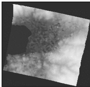
Figure 6. Geo-coded DEM generated from RADARSAT F1-F5 stereo pairs
