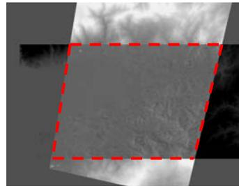
Figure 7. Elevation disparity map calculated as topographic DEM (DTM) from radargrammetric DEM
