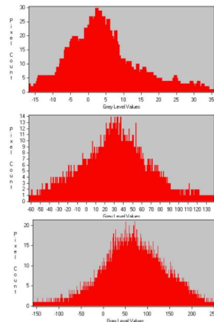
Figure 8. Error histograms for flat, slope and rough topography respectively.
