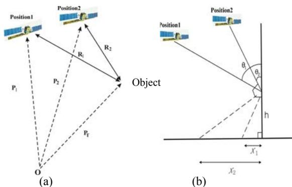
Figure 2. Same Side Stereo SAR Geometry (Min-Ho Ka and Man-Ja Kim., 2001)
