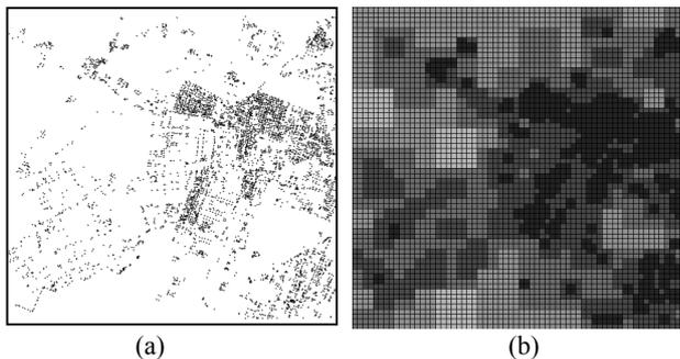
Figure 9. Spatial homologous points distribution (a) and the multi-resolution spline collocation (b)
