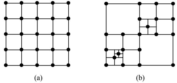
Figure 8. Interpolation grid with mono (a) and multi-resolution (b) approach
