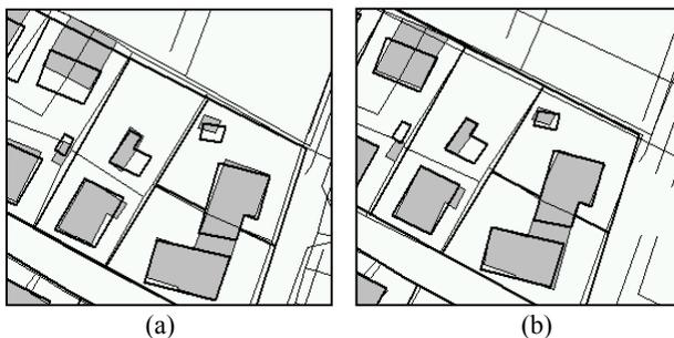
Figure 10. Overlay of two maps using the affine transformation (a) and the multi-resolution spline approach (b)
