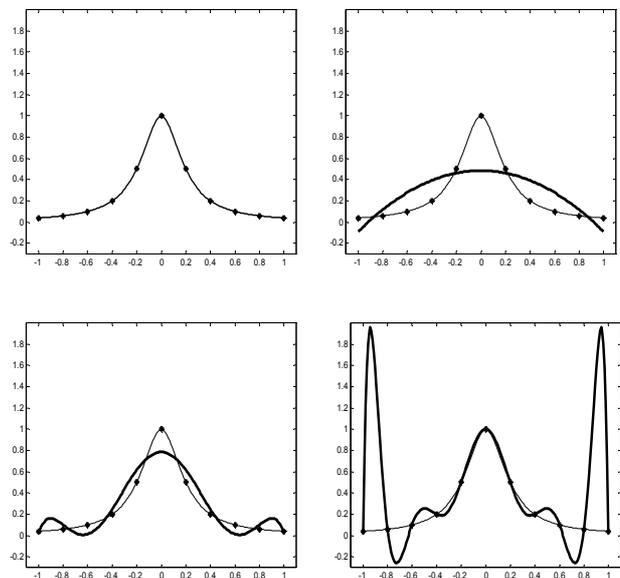
Figure 1. Oscillation problem of polynomial interpolation
