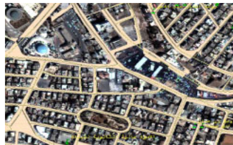
Figure (2): Example in using Ikonos Imagery to validate streets layers built from parcels vector layer.
