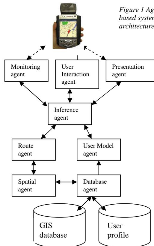
Figure 1 Agent-based system architecture
