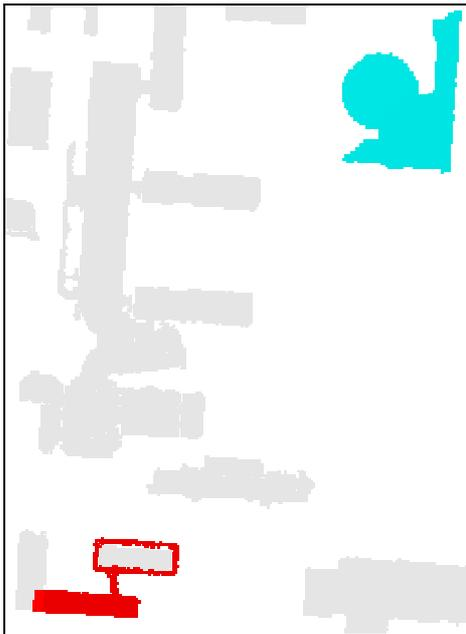
Figure 9: Result of the existing object analyses step of the change detection methodology; light grey: building segments for 2002 DSM, darker grey: new building, dark grey: demolished building
