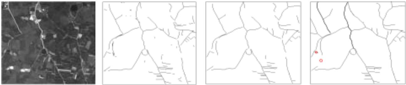
(a) Origin image (b) Central lines after feature grouping (c) Road segments after recognition (d) Detection results
