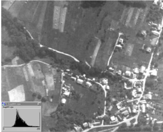
Fig.5. Association of the original image with the image filtered with highpass filter in Fourier space (by addition of two images)
