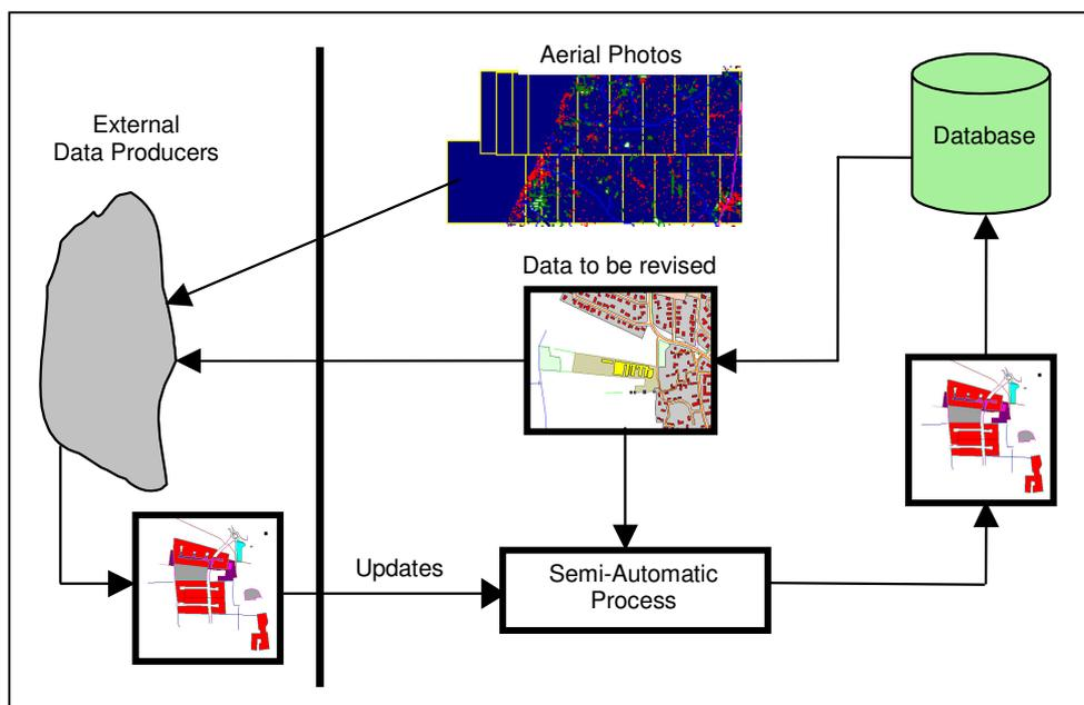
Figure 2. Dataflow for the revision process (after Hoejholt 2004)
