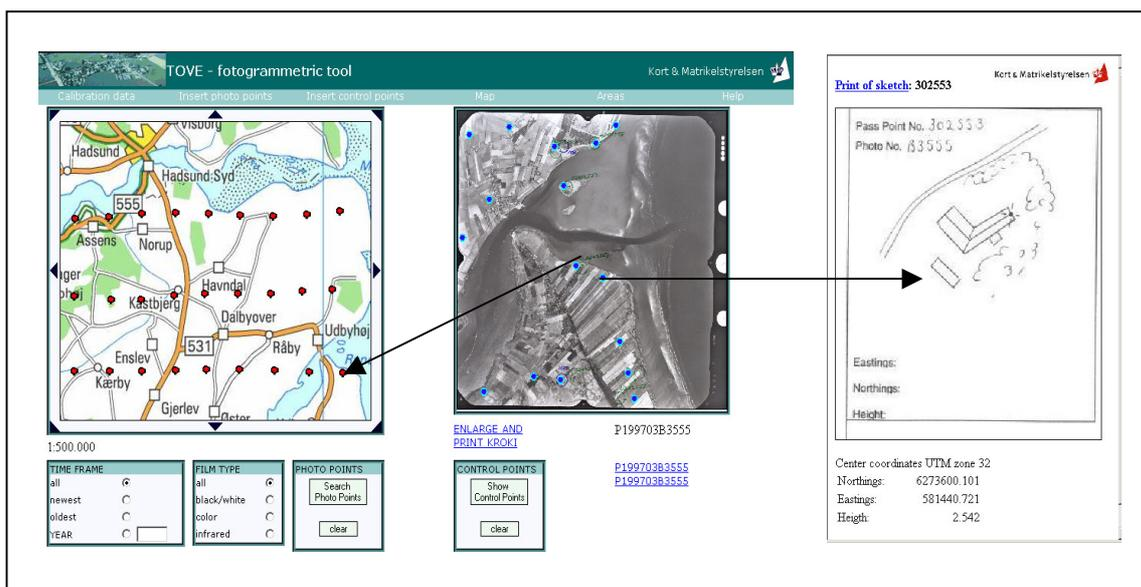
Figure 3. Internet service with ground control and point sketches for photogrammetric revision
