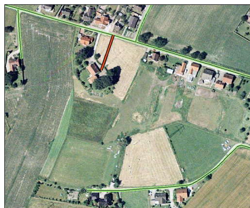
Figure 3. Example for the road verification. Orthoimage, ATKIS DLMBasis, and automatic diagnostics with detected error.
