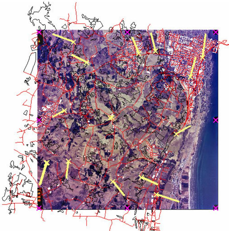
Figure 1. Initial rectification measurement for Vector Transformation. Red crosses are measured fiducials. Yellow crosses are the ground-control-points as vector-object and the yellow connection vectors are pointed to corresponding G.C.P. image pixel. Height differences ( $Z$ ) between GCP's are about 100 meters
