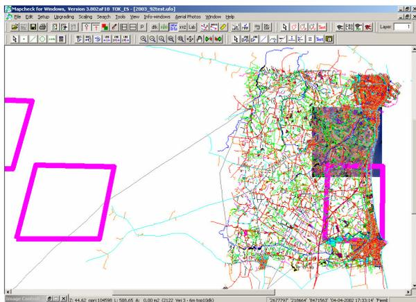
Figure 2. Shown is a block of update-data to be controlled - together with the images, ready for photogrammetric transformation of vector data (X, Y, Z) in that area. Image-coverage are shown with red lines. These are shown photogrammetrically, from the photocenter of the active photo
