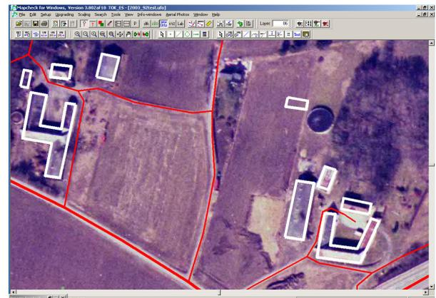
Figure 3. Example of Vector Transformation on raw image. The vector building shown close to silo has wrong Z value (0 m should be 72 m), and is displaced from its correct position by the road.
