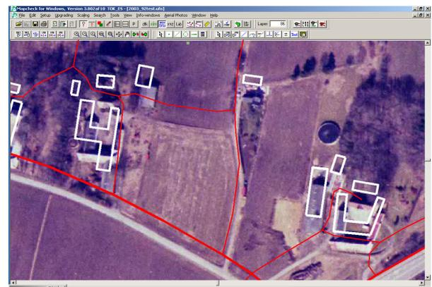
Figure 4. Same area as shown in fig. 3, from the polynomial rectified image (same fiducial and GCP's). Big displacements.
