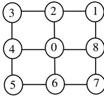
Figure 1 : around a current central position  $(X_0, Y_0)$  with an elevation of  $H_0$ , the neighboring points, having altitudes  $H_1, H_2, \dots, H_8$  are numbered as shown
