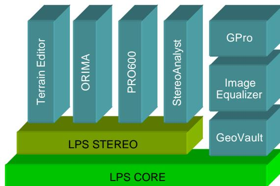
Figure 2: LPS Core and add-on modules
