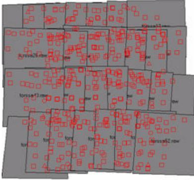
Figure 6a: Graphic overview of the block layout with GCPs, check points and automatically collected tie points
