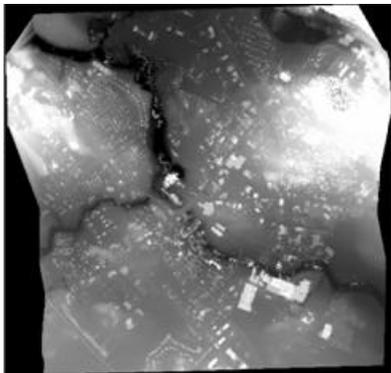
Figure 6b: Automatically extracted DEM for the whole block with grid size 1x1 meters without any editing
