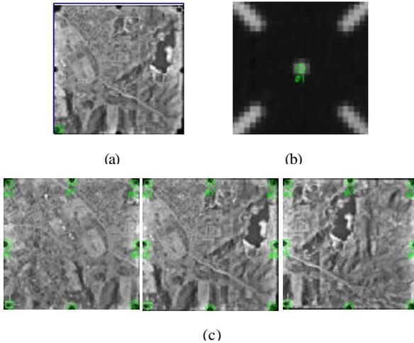
Figure 3: Automatic Fiducial Measurement. (a) Manually measure one fiducial mark, (b) Automatically measured fiducial Mark with least square template matching, (c) All automatically measured fiducial marks in a strip.
