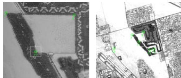
Figure 4c: Enlarged view of three found tie points in their original scale and orientation
