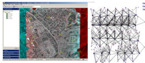
Figure 5: ORIMA stereo point measurement interface and graphic point and image connection display
