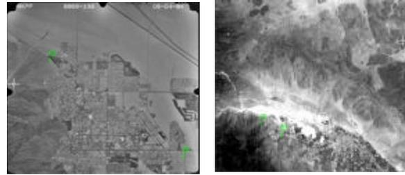
Figure 4a: A registered aerial image (left) and a raw SPOT image (right) with 2 manual tie points
