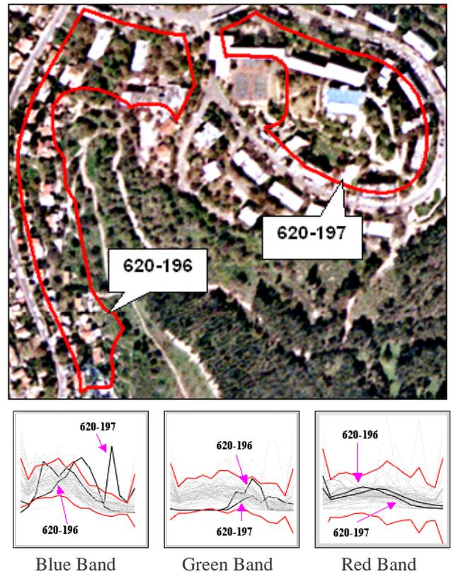
Figure 2. Results for two discrepant polygons of “natural forest” and their spectral signatures for the RGB bands of a Color Orthophoto.
