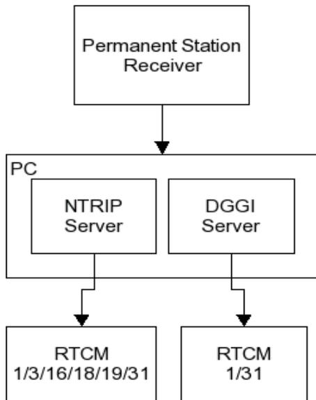
Figure 3. Scheme of The Permanent Station with the RTCM Servers
