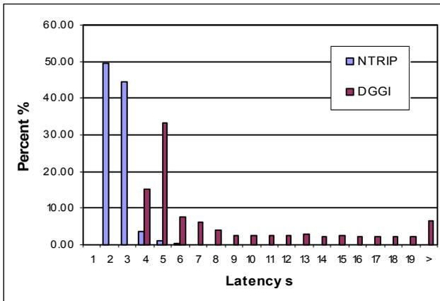
Figure 5. NTRIP-DGGI server comparison
