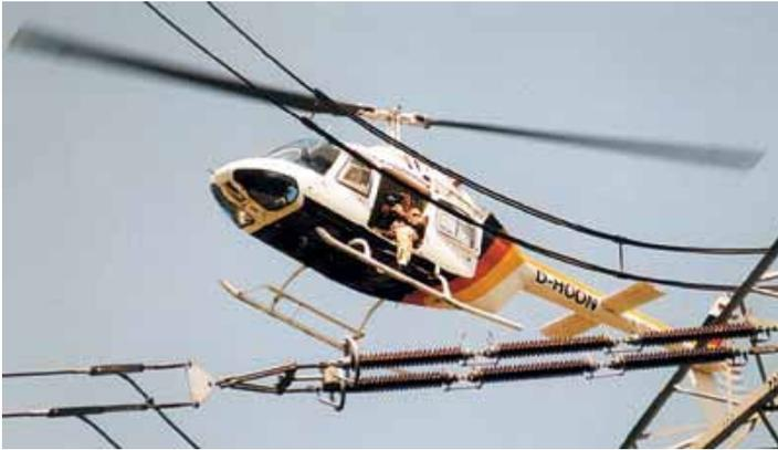
Figure 8: photo of a helicopter of the company Rotorflug GmbH during an inspection of powerlines, already operation with an AeroLogger system
