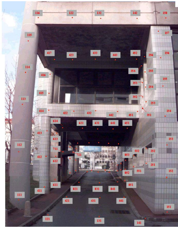
Figure 2: Calibration polygon test field. 75 materialized GCP have been measured with an accuracy of 0.1 mm.
