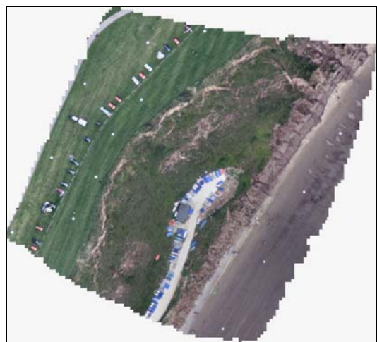
Figure 1. Orthophoto of Filey Bay test site, taken using DCS 660. Area is approximately 200 x 200 m
