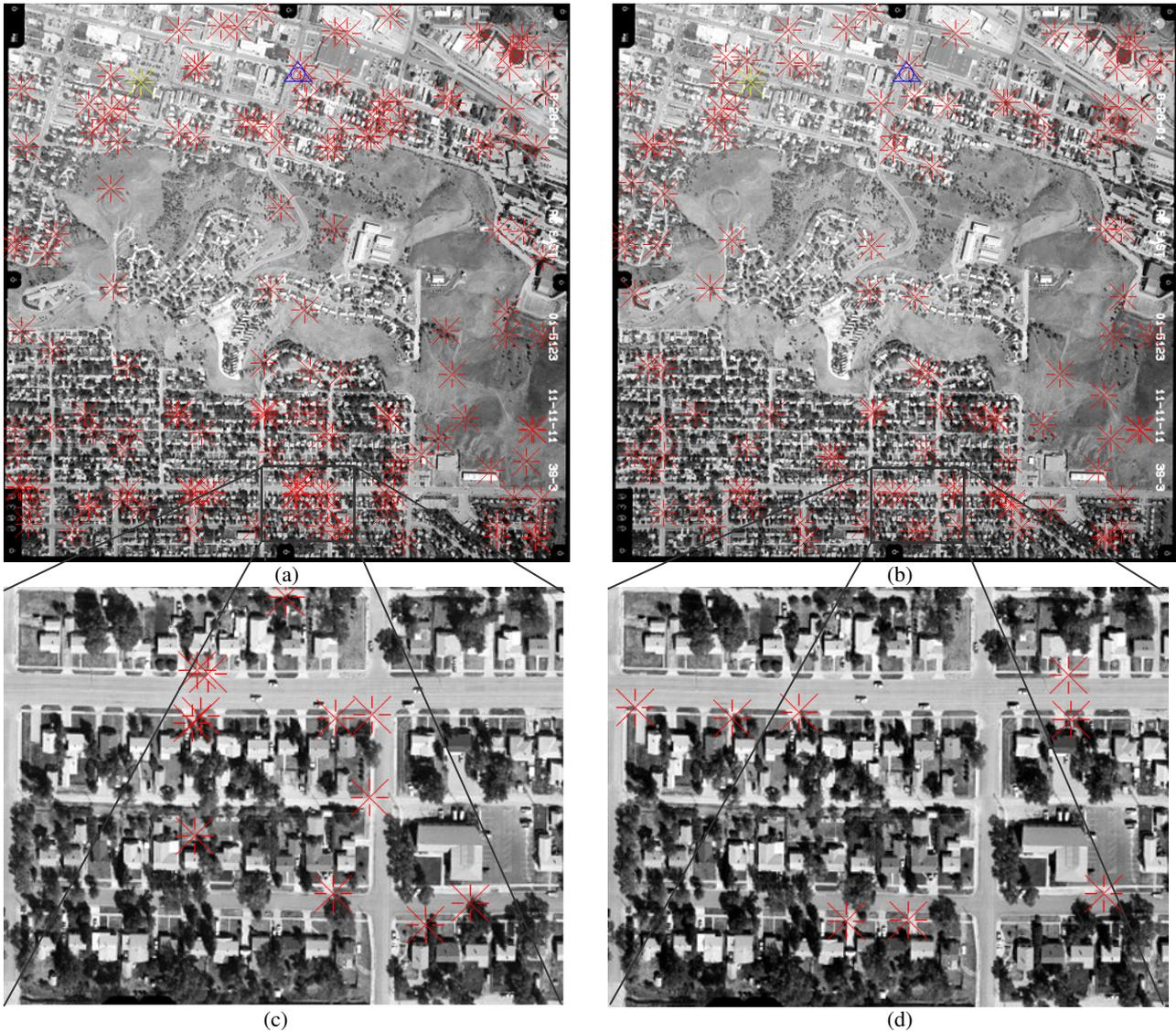
Figure 4. Automatically generated Tie/Pass Points (a), (c) extracted tie/pass points before removal of shadow points, (b), (d) extracted tie/pass points after removal of shadow points
