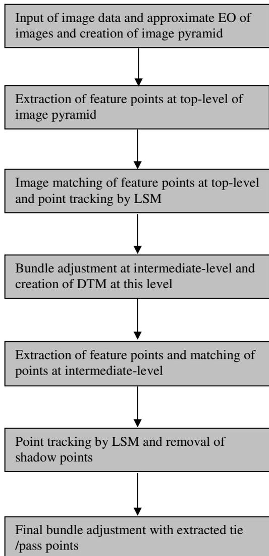
Figure 1. Automatic Generation of Tie/Pass Points in Z/I Imaging's ISAT
