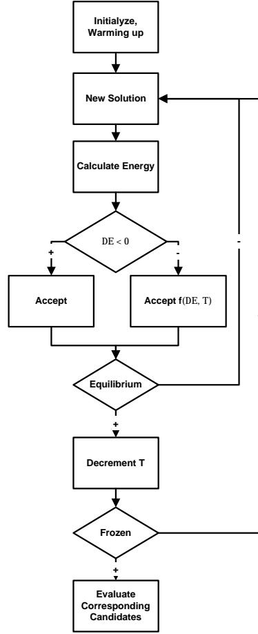
Figure 6: Principle of the metropolis algorithm
