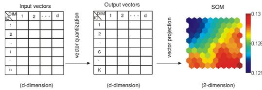
Figure 1: Illustration of SOM principle
