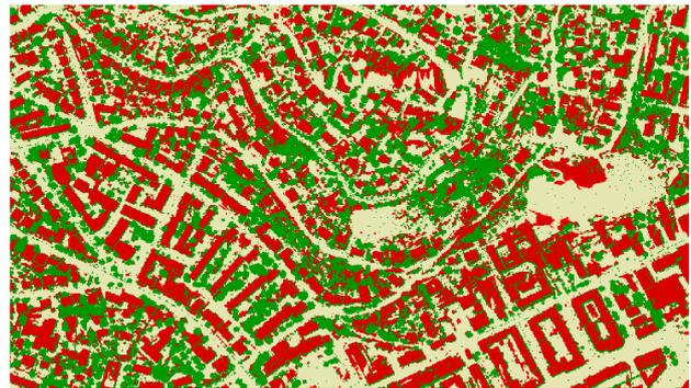
Figure 4.2 - Results of the final classification using the road method, site No. 1.
