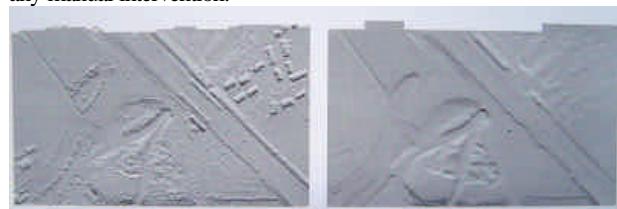
Figure 4 Surface interpolated using the original data. DHM derived by the filtered data.
