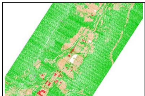
Figure 3. LIDAR points after manual edition.
