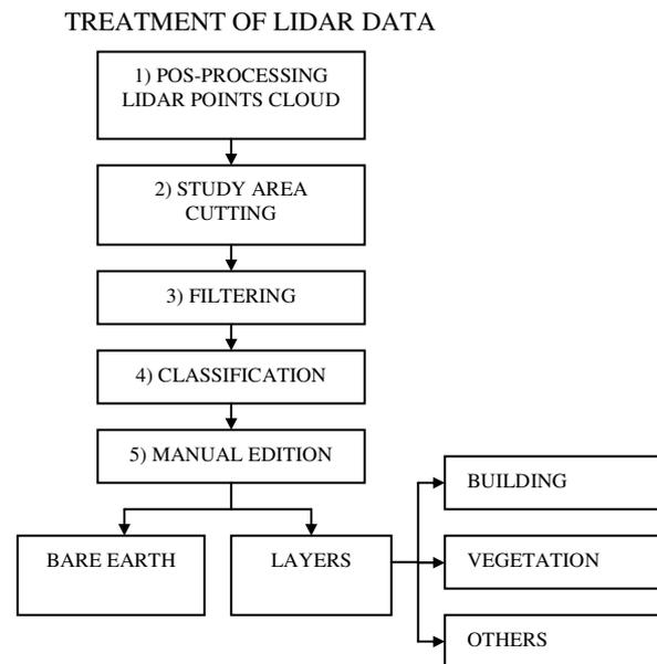
Figure 2. Flow chart of LIDAR data treatment.
