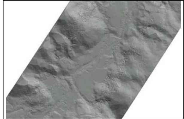
Figure 5. Part of DTM generated from LIDAR points.
