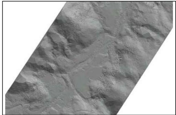
Figure 5. Part of DTM generated from LIDAR points.
