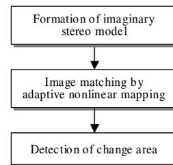
Figure 2. Process flow of 2D image matching method
