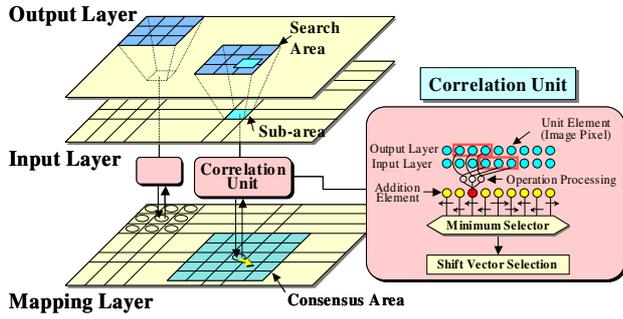
Figure 5. Conceptual diagram for adaptive nonlinear mapping
