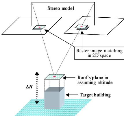
Figure 8. Process flow of indirect comparison method
