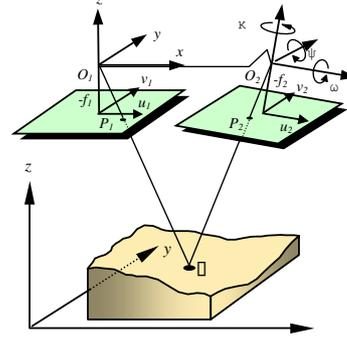
Figure 4. Coordinate system in a stereo model
