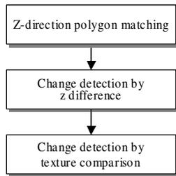
Figure 7. Process flow of 3D image matching method
