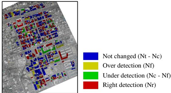
Figure 13. Change detection by 3D image matching method
