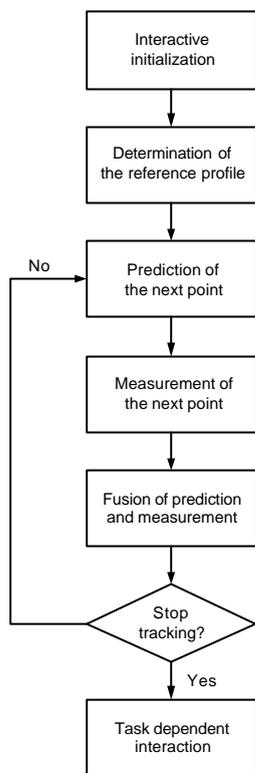
Figure 5. Flow chart of the line following algorithm
