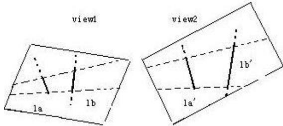
Figure 4: epipolar constraint
