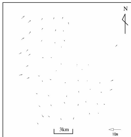
Fig.6 Horizontal component of error vectors
