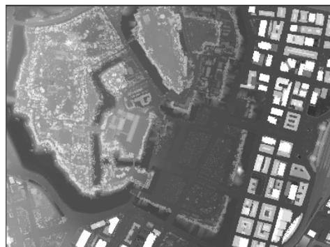
Fig. 13 DSM from aerial laser scanner
