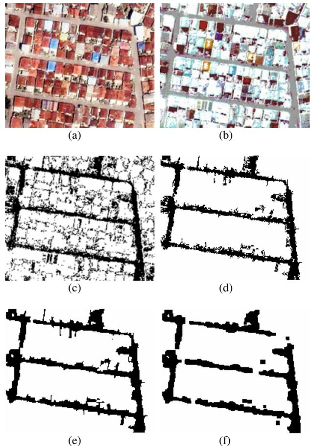
Figure 6. Road extraction from pa-sharpened IKONOS image of a rural area of *Kish* island: (a) original image, (b) fuzzy classified image, (c) segmented image, (d) result of trivial opening, (e) initially identified road surface, (f) result of opening operation
