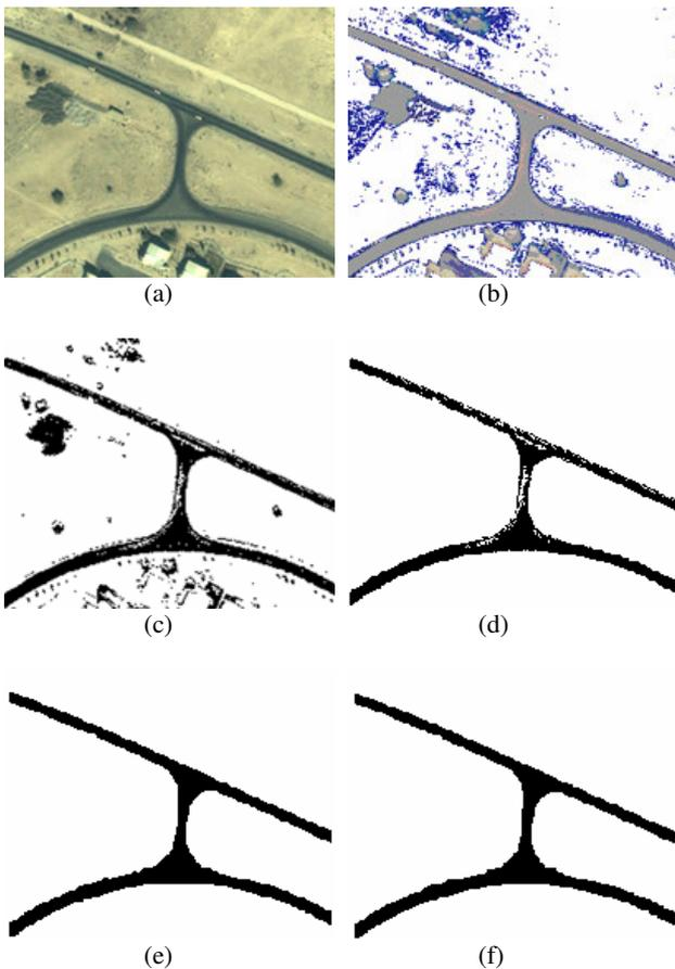
Figure 5. Road extraction from pan-sharpened IKONOS image of a rural area of *Kish* island: (a) original image, (b) fuzzy classified image, (c) segmented image, (d) result of trivial opening, (e) initially identified road surface, (f) result of opening operation
