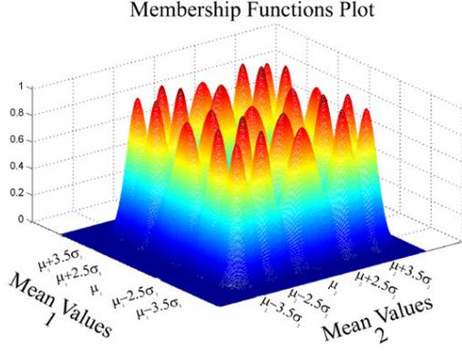
Figure 1. Defined classes using MFs of bands 1 and 2
