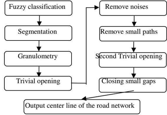
Figure 3. Block diagram used in morphology approach
