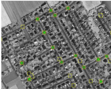
Figure 5. Detected road junctions. Boxes show initial detection. Crosses show detection after filtering with flat spot criterion.
