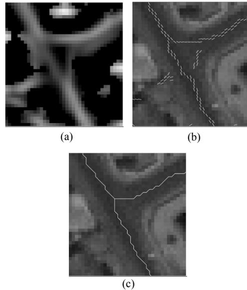
Figure 6. Detail of the information content of a junction in very-high resolution. (a) maximum eigenvalue, (b) direction vectors of detected ridge pixels, (c) thinned response after region growing.
