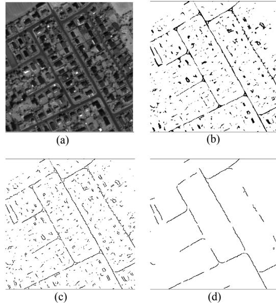
Figure 2. Example of ridge detection. (a) original, (b) detected ridge pixels, (c) thinned result, (d) filter on minimal segment length.
