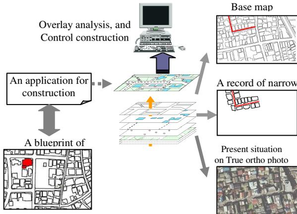
Figure 2: Image of using fundamental data for the construction control at the narrow road areas
