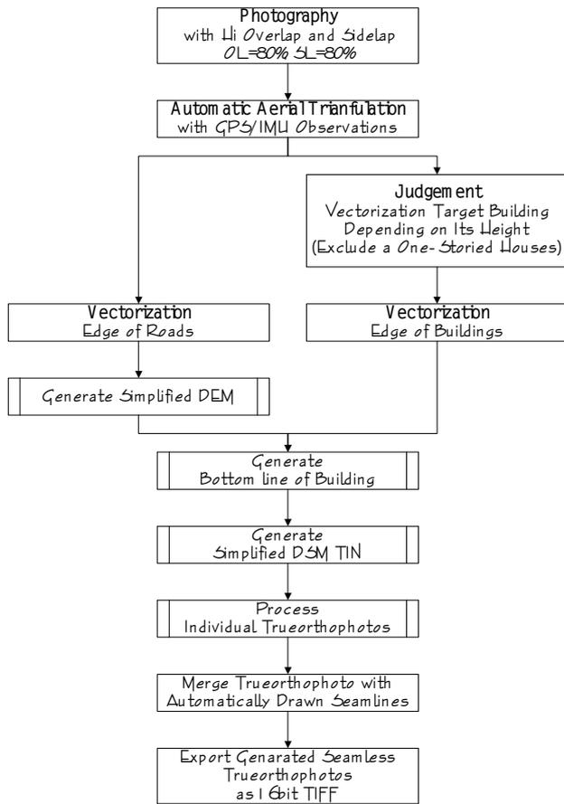
Figure 5. Flowchart of True orthophoto generation method
