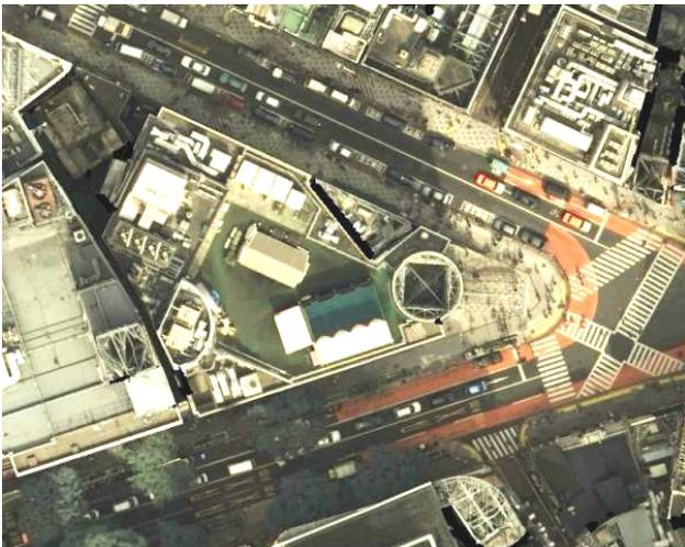
Figure 9. Generated true orthophoto same area as figure 8
