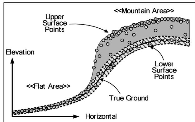
Figure 1. Principle of Filtering Method
