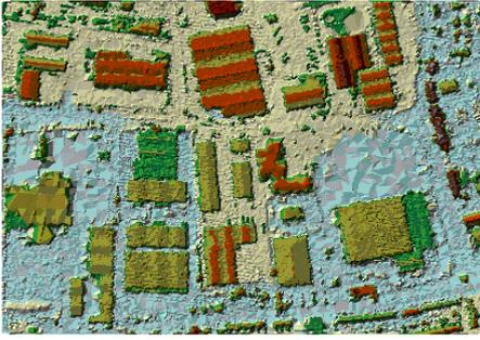
Figure 2. Greenwich lidar DSM
