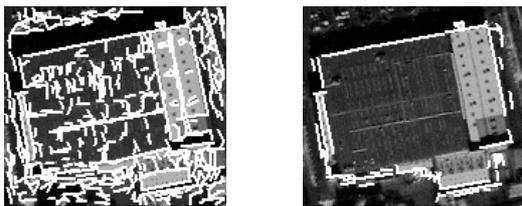
(a) extracted straight lines (b) filtered boundary lines
