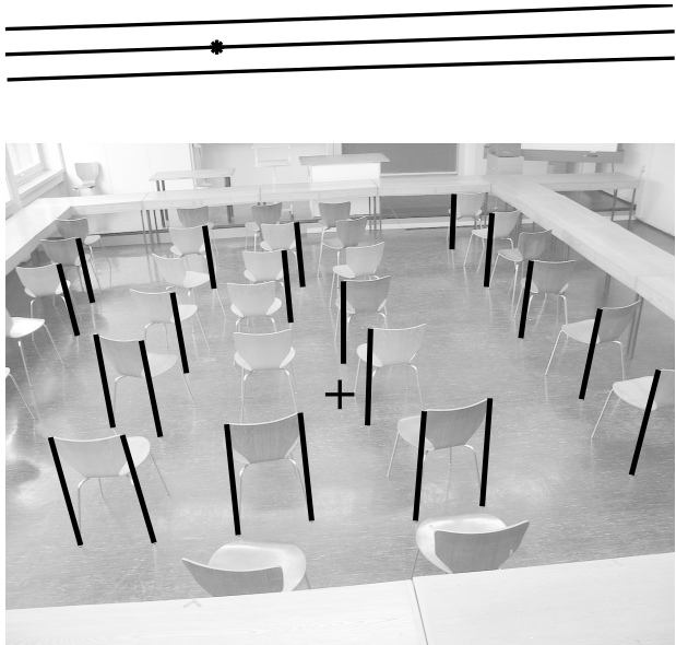
Figure 3: shows the observed corresponding foot and head points as well as the estimated horizon line, its point of gravity and its hyperbolic error band ( 3\sigma intervals).
