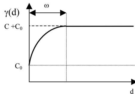
Figure 3. A hypothetical semivariogram.  $C_0$  – a local variability in the scale of a single sample, so-called the nugget effect;  $C$  – the sill value;  $\omega$  – the influence range;  $d$  – distance (lag);  $\gamma(d)$  – semivariance
