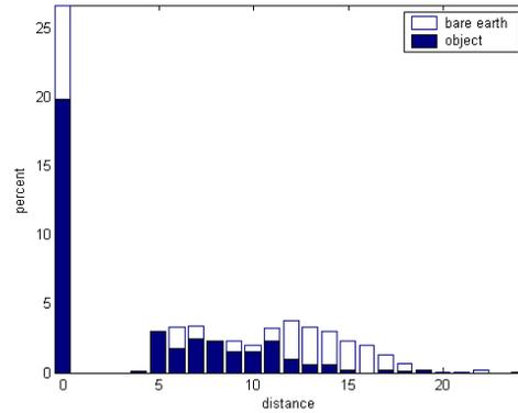
Figure 10. The relationship between the first-last impulse distance, and the type of surface (bare earth, object) for forest area
