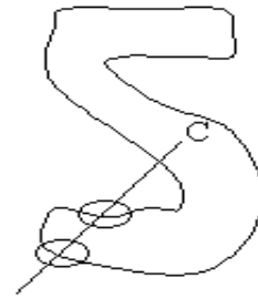
Figure 4: A non convex object. The procedure fails on the straight line segment shown on this figure. It will not detect the border points marked with a circle.
