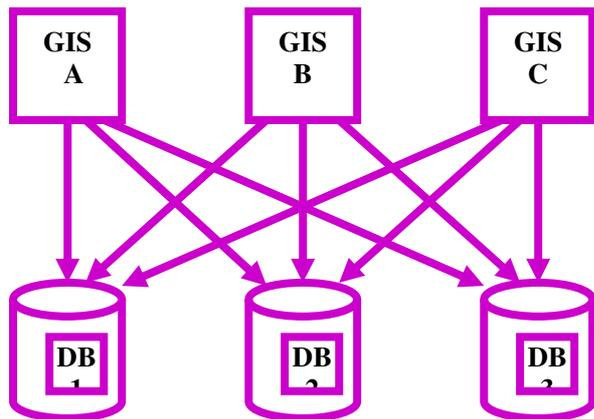
Figure 1 Interoperability Based on Direct Access to Databases
