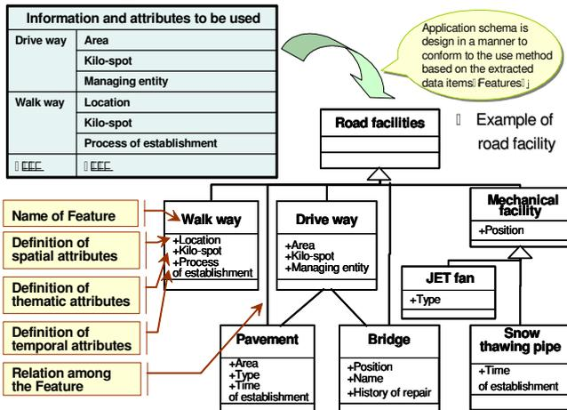
Figure 5. Design of application schema
