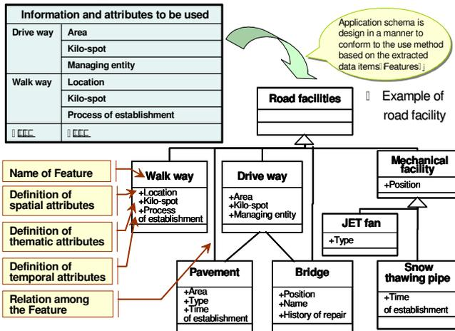
Figure 5. Design of application schema
