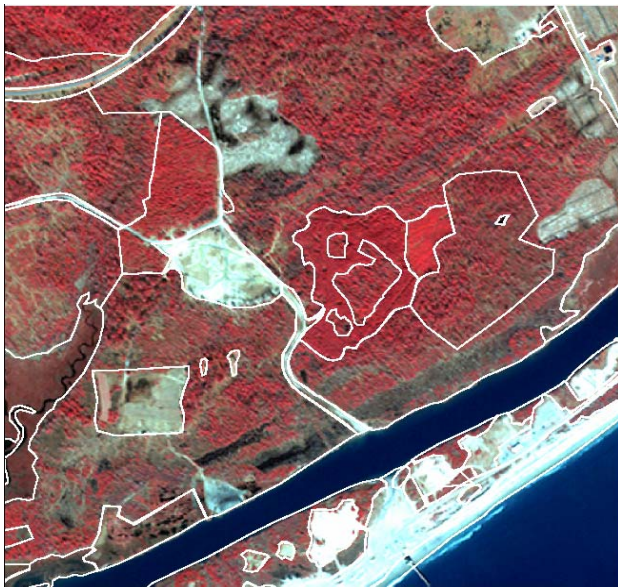
Figure 2. IKONOS multispectral image (2048 x 2048 subset) of the Camp Lejeune study site overlaid with vector GIS information
