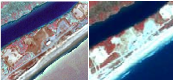
Figure 7. The subset of the GIS enhanced image (left) shows a higher level of detail compared to the globally enhanced image (right) (contrast stretch with \pm 2\sigma )
